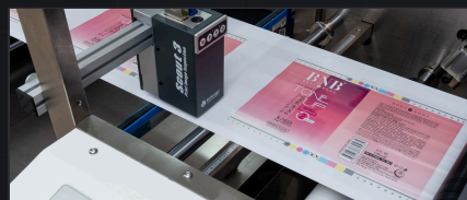
FIG.05 Vision Camera Inline vision camera and monitor for on-screen register inspection.
