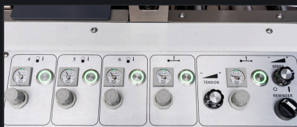
FIG.04 Pneumatic Control · NIP Roller Pneumatic control of the nip-roller pressure.
