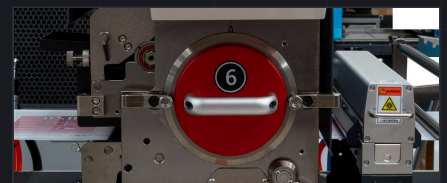
FIG.06 Printing Station Easy plate-cylinder change design.
